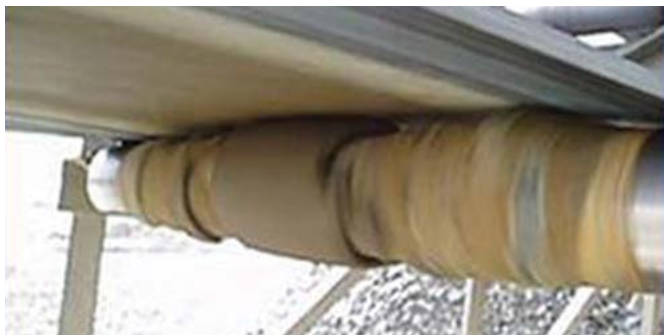
Carryback material buildup on a steel roller
