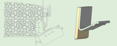
Designed for longer life sealing at the harshest transfer/feed points, Smiley Monroe introduces its new energy-saving, low friction primary 65° and secondary 75° shore A hardness polyurethane (PU) conveyor skirting.
